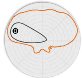
Figure 5. T750 5GHz Elevation Antenna Patterns
